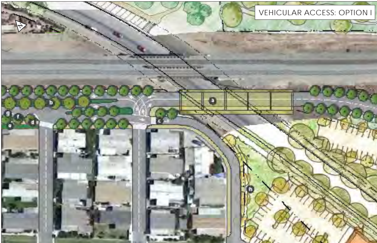
Figure 3.5 Optional Street Alignments for New Vehicular Access to the Railroad Parcels. Option 1: Build a bridge over Front Street. Option 2: Build an automobile underpass extending from Kidder Street in a u-shape. Option 3: Build an underpass from the railroad parcels to the agricultural fields northeast of the tracks, eventually emerging with San Vicente Street.
