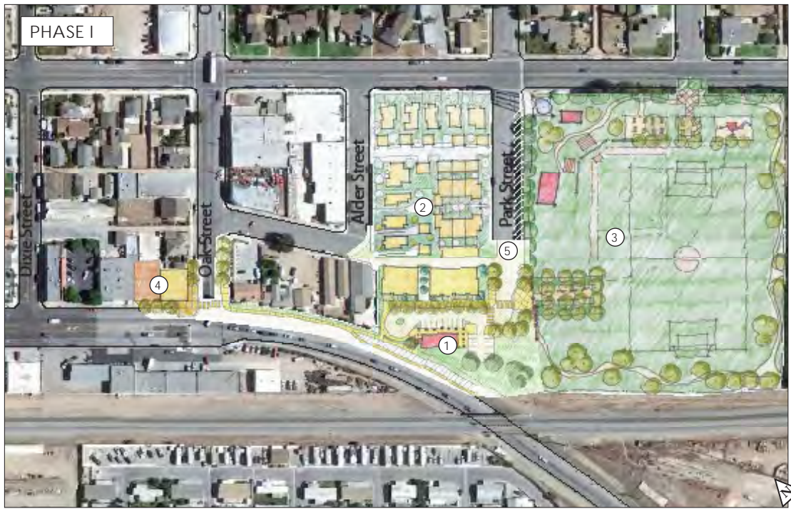
Illustrative site plans of two phases of development for the Vosti Park area. Proposed improvements for Phase I include 1) relocation of the City Yard and a new community center, 2) medium and high-density residential developments, 3) park enhancements and additional street trees, 4) infill development on the corner of Oak and Front Street, 5) reconfiguration of the two smaller blocks between Alder and Park Streets into one large block and closing off vehicle access between Alder Street and Park Street, and 6) a pedestrian-only path connecting Vosti Park to Alder Street through the proposed residential development.
