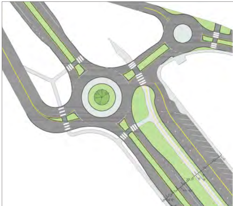
Figure 3.6 Sample Design of a Modern Roundabout
