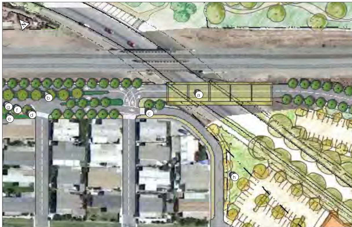
Close-up plan drawing of proposed location and design for automobile bridge over Front Street and the railroad tracks. The bridge will provide access to the railroad district from the South Gateway area.
